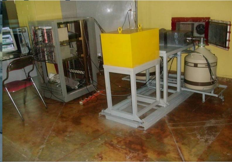
Gamma-gamma coincidence spectroscopy
