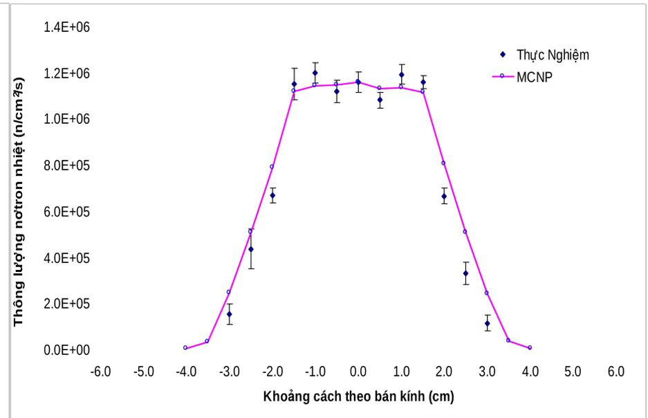
Monte-Carlo simulation and experiments for radial distribution of thermal neutron fluxes
