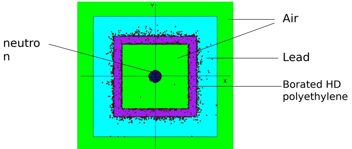
Monte-Carlo simulation for filtered neutron beam at Dalat research reactor
