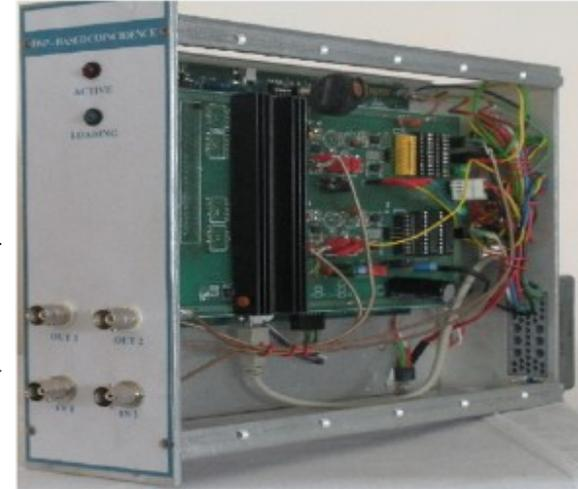
The integrated coincidence spectroscopy (2M size), using FPGA and DSP
