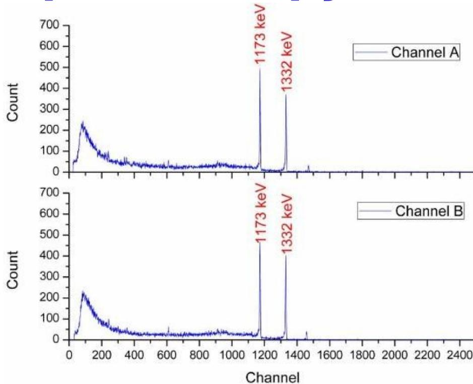
Energy spectrum of both detectors. Energy resolution is better 12% at 1332 keV (Co-60), slightly better than our current analog one.
