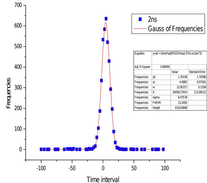
Coincidence curve. Timing resolution is ~13 ns (compared to 10 ns with the current analog one).
