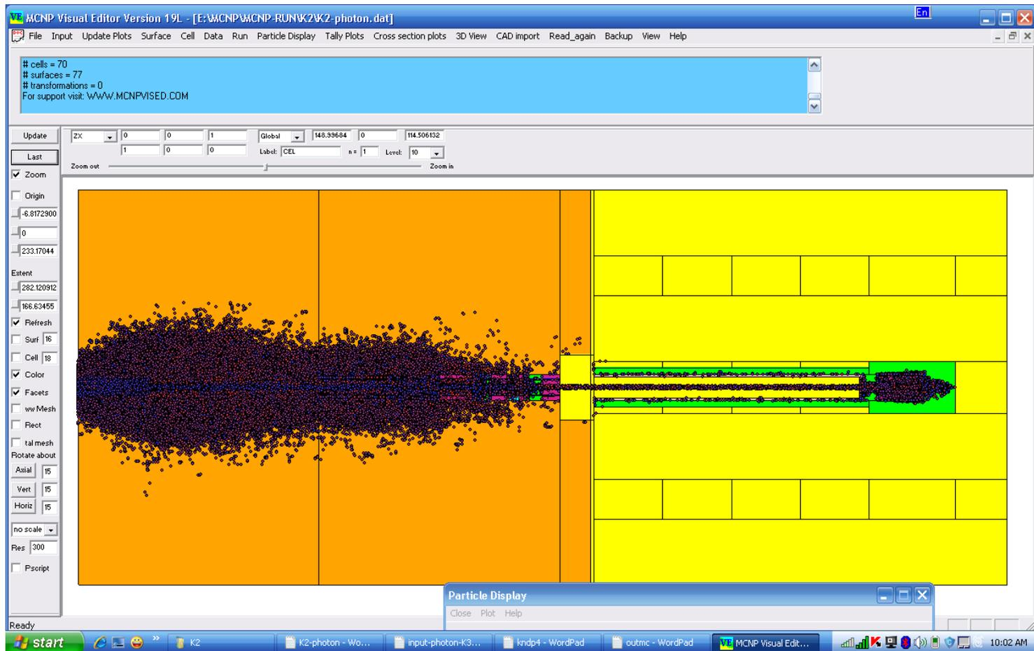
Monte-Carlo simulation of gamma radiation for filtered thermal neutron beams at Dalat research reactor
