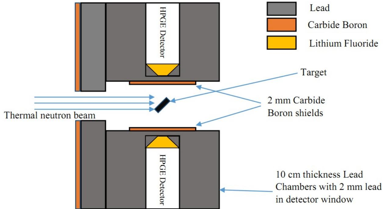
Neutron flux at target position =  $1.7 \times 10^5 \text{ n.cm}^{-2}.\text{s}^{-1}$
