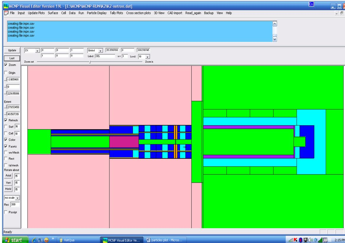
Monte-Carlo simulation and design for filtered thermal neutron beams at Dalat research reactor
