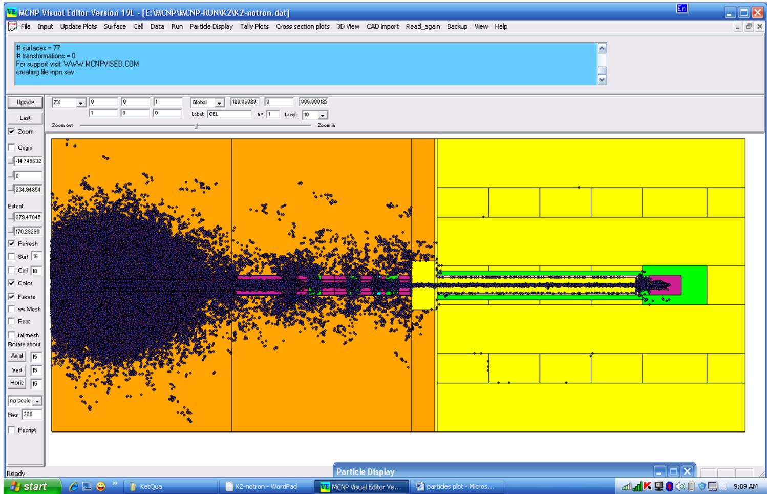
Monte-Carlo simulation of neutron radiation for filtered thermal neutron beams at Dalat research reactor
