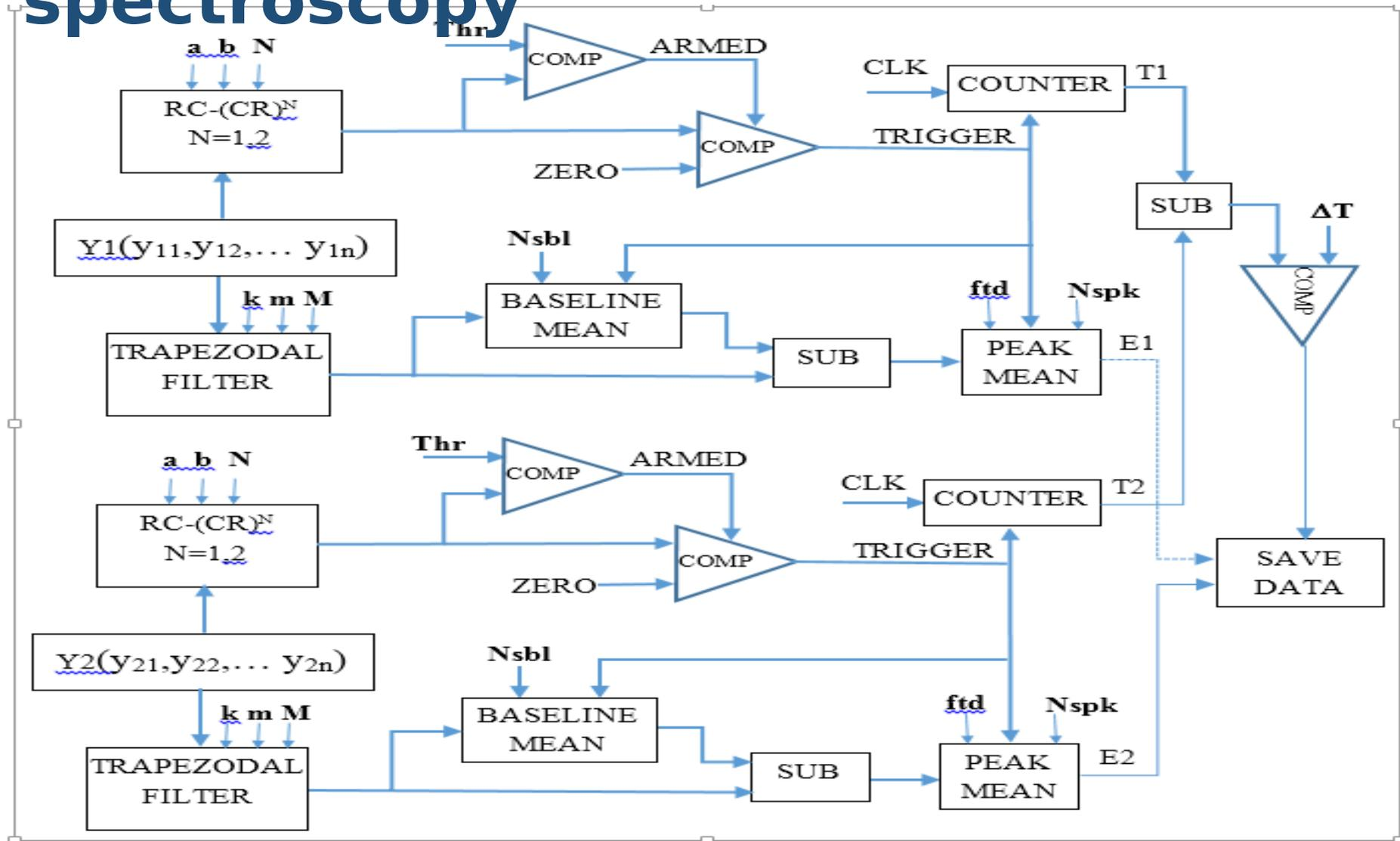
Coincidence spectroscopy design based on DSP
