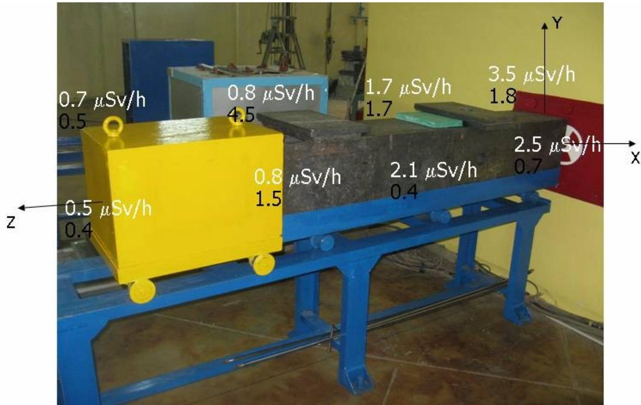
An outside view of filtered neutron beam at the channel No.2 of Dalat research reactor with radiation dose rate information (white color for neutron and black color for gamma)
