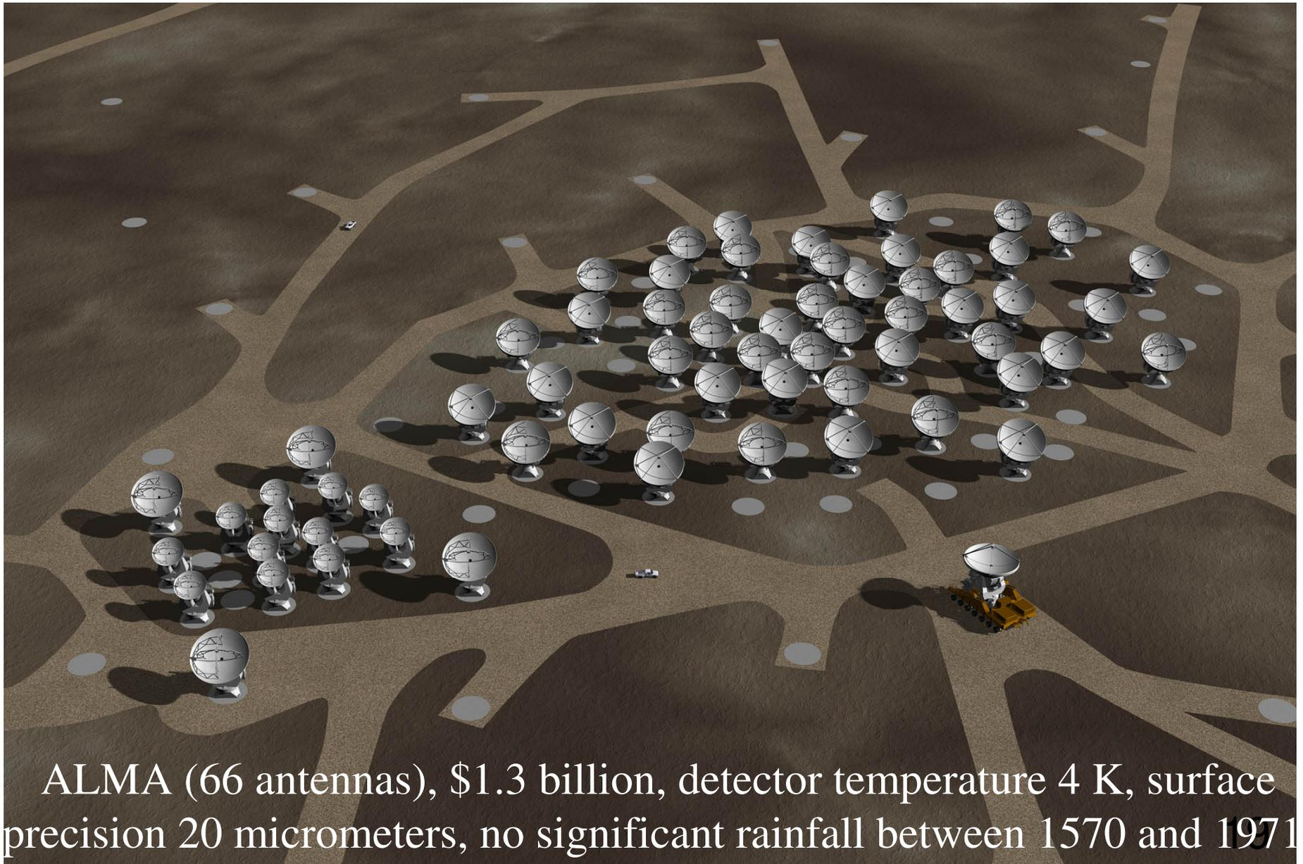
ALMA (66 antennas), \$1.3 billion, detector temperature 4 K, surface precision 20 micrometers, no significant rainfall between 1570 and 1971
